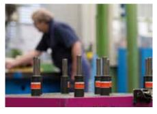
parts are produced in each stroke here. Production is carried out in our AEF press shop on a servo press with a pressing force of 6,300 kN.
